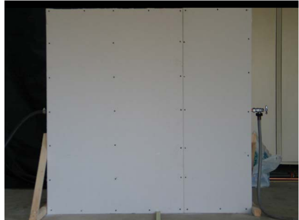
Figure 2 – Test wall after installation of sheet rock
